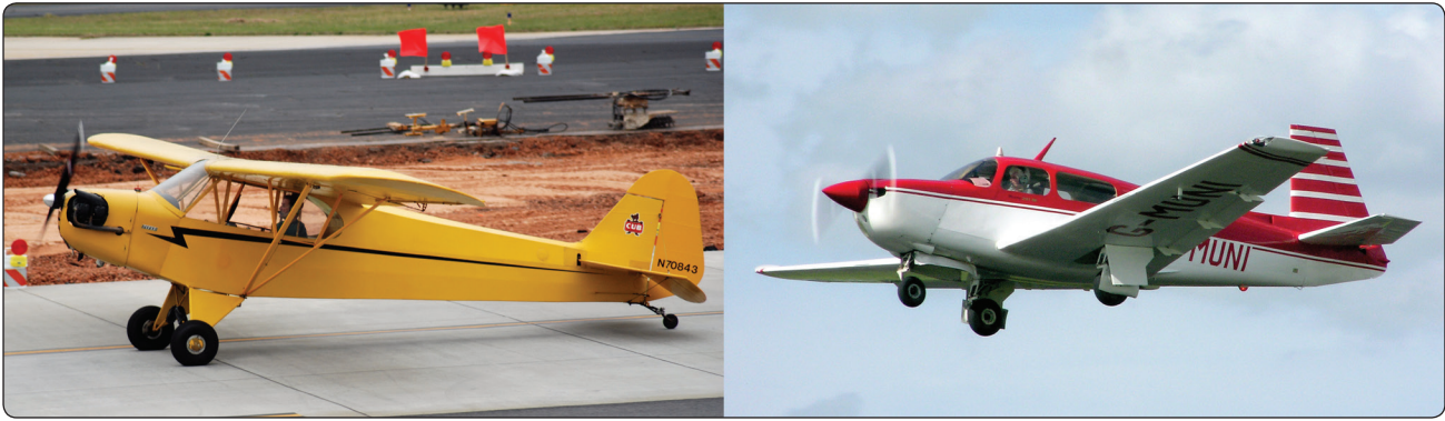
Figure 13-1. The Piper Super Cub on the left is a popular tailwheel airplane. The airplane on the right is a Mooney M20, which is a nosewheel (tricycle gear) airplane.
