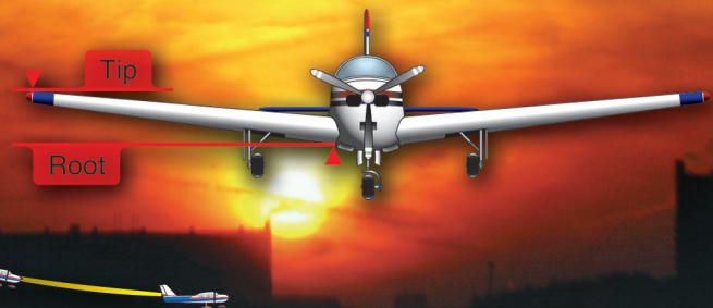
Wing Washout Wing root has greater angle of incidence than wing tip.
