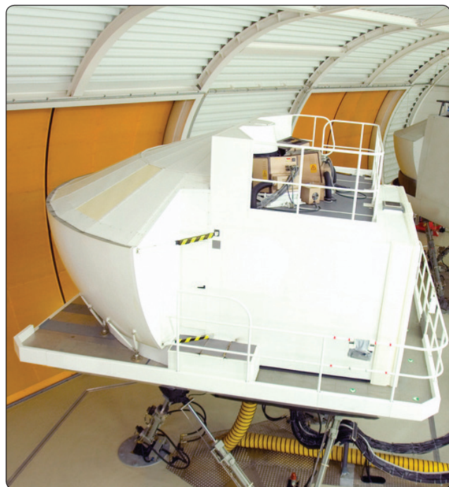
Figure 4-17. A Level D full-flight simulator could be used for UPRT.
